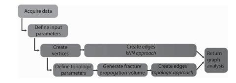
Figure 3 Workflow for preforming a graph analysis to spatially assess induced fractures.
