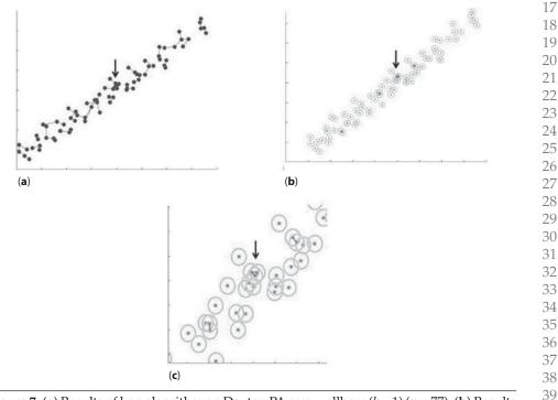
**Figure 7** (a) Results of knn algorithm on Dayton PA area wellbore (k = 1) (n = 77); (b) Results of topological algorithm on Dayton PA wellbores (n = 77); (c) Results of topological algorithm on Dayton PA wellbores, zoomed in on wellbores associated with leakage. Black arrows point to overpressurized wellbore. All results are shown in 2D form for clearer visual representation of results.
